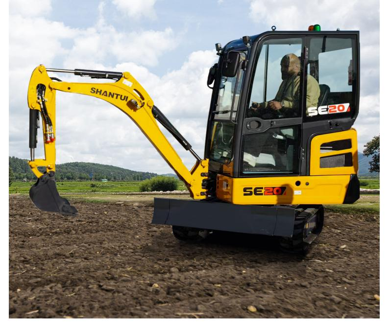
Engine model: Engine power: Operating weight: Bucket capacity: Kubota D902 11.8kW/2300rpm 2000kg 0.04m<sup>3</sup>
